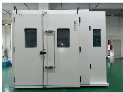
3.6 m3 constant temperature and humidity laboratory
