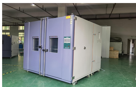
3.6 m3 constant temperature and humidity laboratory
